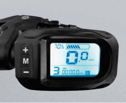
Everything under control: A functional, complete and legible LCD dashboard allows you to keep under control every function, from speed to travel time, from partial to total kilometers, from the remaining battery charge to the selection of the pedal assistance steps.
