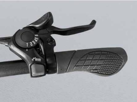
Featuring six-speed transmission, rear derailleur, Shimano Tourney TZ has been designed with e-bike lovers in mind. This gearbox installed on the S9 allows us, in fact, to perfectly adapt the selected ratios to the slope of the road and to our physical condition. In this way, it will be really simple to adjust the pedaling power by optimizing it to the path we are about to take.
