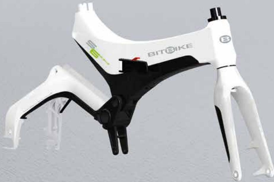
The frame material is magnesium alloy, which is 1/3 lighter than aluminum alloy and has better impact resistance. The frame process adopts magnesium alloy die casting technology, which breaks the traditional welding process and ensures that the whole electric bicycle has no welding.
