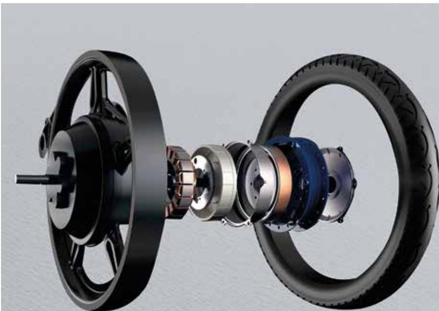
Electric hub motor: it is a motor positioned in the rear hub of the bicycle. This position offers the best weight balance by compensating that of the battery on the front. This engine is ideal for overcoming uphill slopes of around 10-15% and has a lower consumption in the plains than other similar engines on the market. The power of 250Watt at 36 Volts allows a maximum speed of 25Kmh with a torque of 12Nm. The autonomy that you have in optimal conditions with a charged battery is 55Km.
