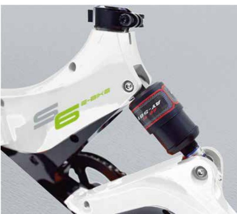
The ride comfort of this bicycle is guaranteed by the rear shock absorber which absorbs the roughness of the road. Even on the most bumpy roads it will always be comfortable to use the bike together with maximum road holding.
