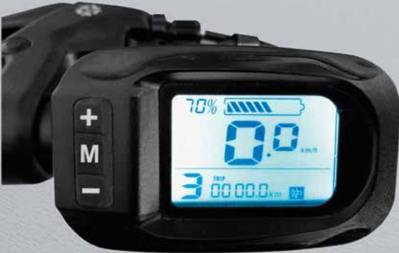
Everything under control: A functional, complete and legible LCD dashboard allows you to keep every function under control, from speed to travel time, from partial to total kilometers, from the remaining battery charge to the selection of the pedal assistance steps.
