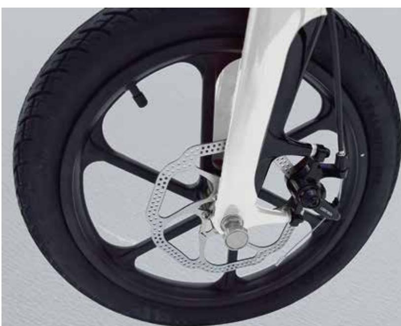
Safety in mind: The braking distances of a vehicle are essential for safety, and therefore this bike is equipped with a front and rear disc brake with mechanically operated caliper. This type of brake allows limited stopping distances in all conditions. The conformity of the daisy disc in addition to the aesthetic factor allows a greater dissipation of heat and dust that is created on the braking surface of the disc.
